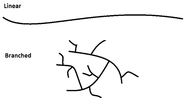
Fig. 1 Linear versus branched polymers. Drawings representing linear and branched polysaccharides. Viscosity is a function of the volume of a molecule as it rotates in water (effective hydrodynamic size), so the longer the straight chain, the greater the effect the linear fiber can have on viscosity. The volume “swept out” by a fully extended linear fiber is much greater than a fiber with the same molecular weight but with a “bush-like,” highly branched configuration
